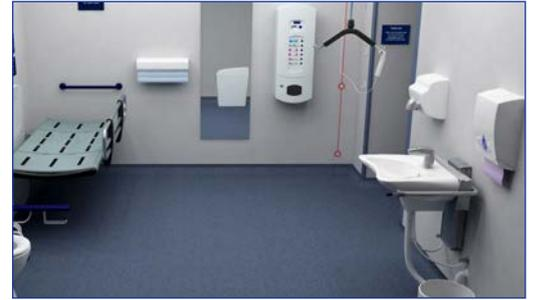
The floor of the accessible toilet should be a high contrast solid colour to the walls, to create a clear distinction of the edges of the facilities.
