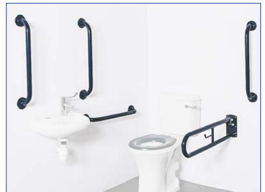
Grab rails must be wall-mounted vertically, diagonally at 15 degrees, and horizontally, with at least one drop-down grab rail on either side of the toilet for left and right-hand transfer.
